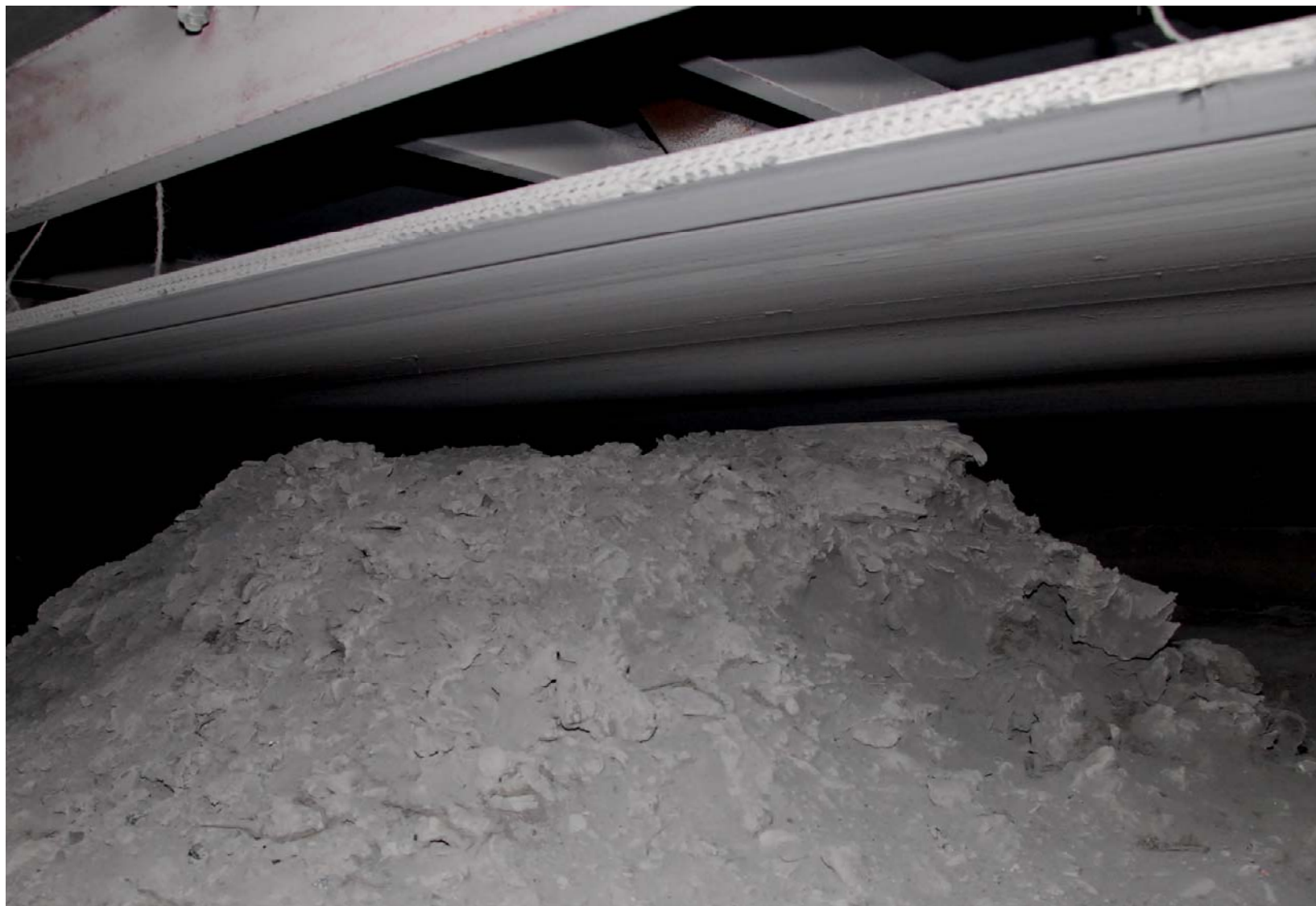
Figure 8. Accumulations of loose coal with the top of the pile flattened due to rubbing the moving belt.
