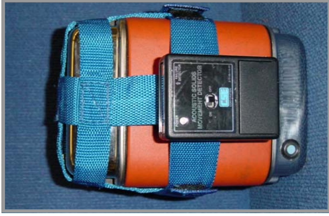
Acoustic Solids Movement Detector Mounted on a SR-100
