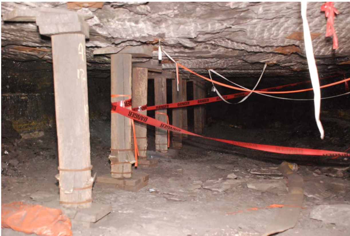
Figure 4. Photograph of Tailgate 1 North No. 7 entry showing only one row of posts installed. The approved roof control plan required two rows of 8' cable bolts or posts.
