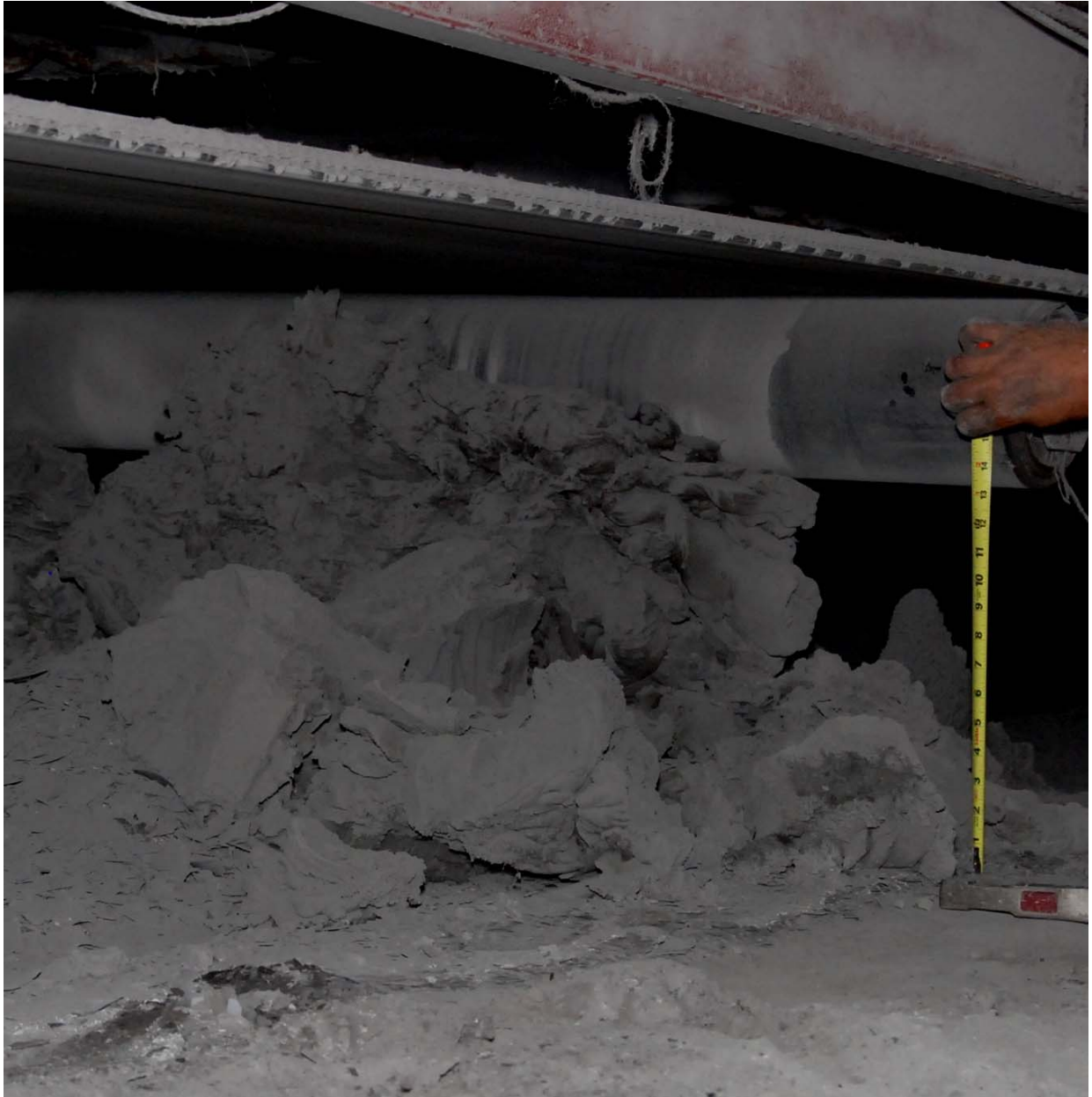
Figure 9. Accumulations of loose coal built up to the point that the belt roller is turning in the accumulations.
