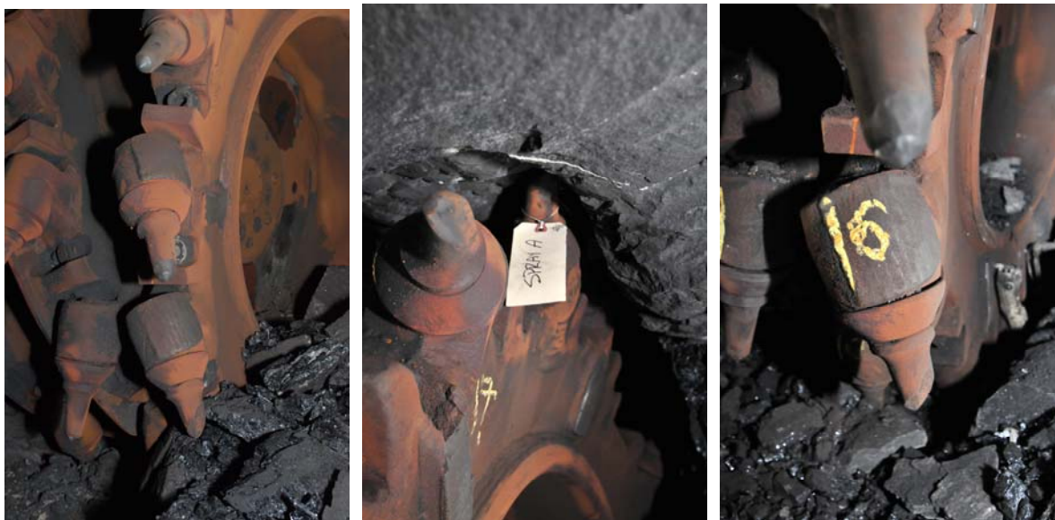
Figure 30. 1 North Panel tailgate drum, showing configuration of water sprays used in the pick-point flushing system. Note that sprays are directed toward the front of the bits, one missing water spray, and two bits exhibiting extreme wear.
