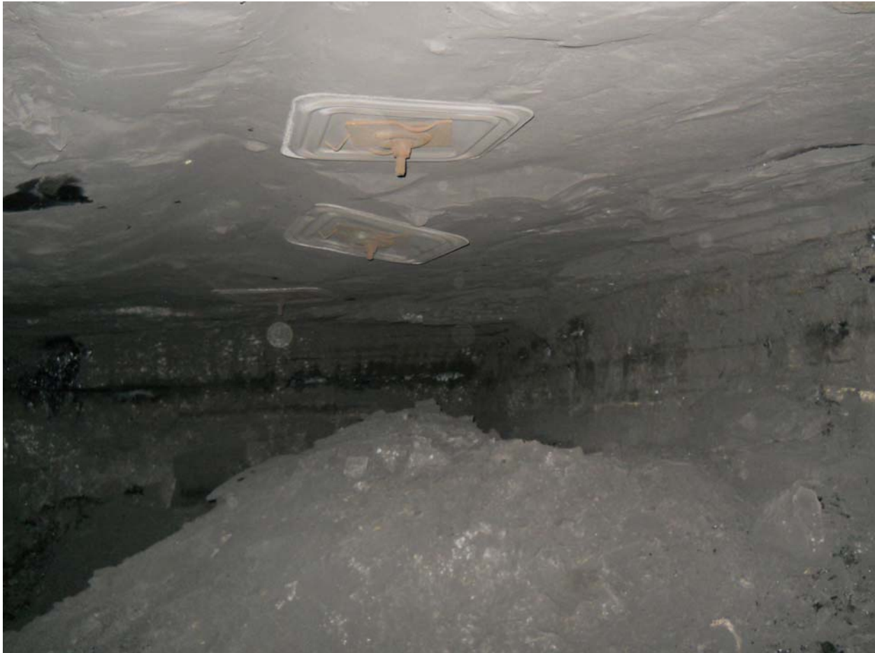
Figure 3. Accumulations of loose coal, coal dust, and float coal dust were measured up to 7 feet wide by 12 feet long by up to 4 feet in depth. These were found consistently along every single air course.
