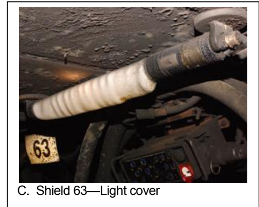
Figure 8. Except for the headgate and tailgate regions, coked dust inside the longwall was found only between shield 41 and shield 72, together with other indicators showing evidence of flame and heating at this location. (A larger map can be found in Appendix 7.9-1, Map 4 ).
