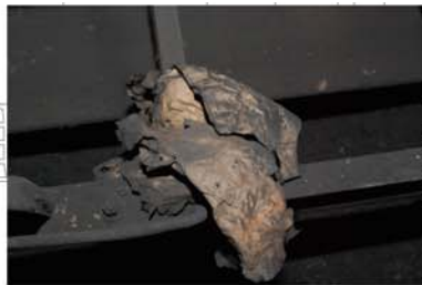
EXAMPLE OF "FINAL FORCES"-- PAPER LOOSELY CAUGHT ON BELT STRUCTURE
