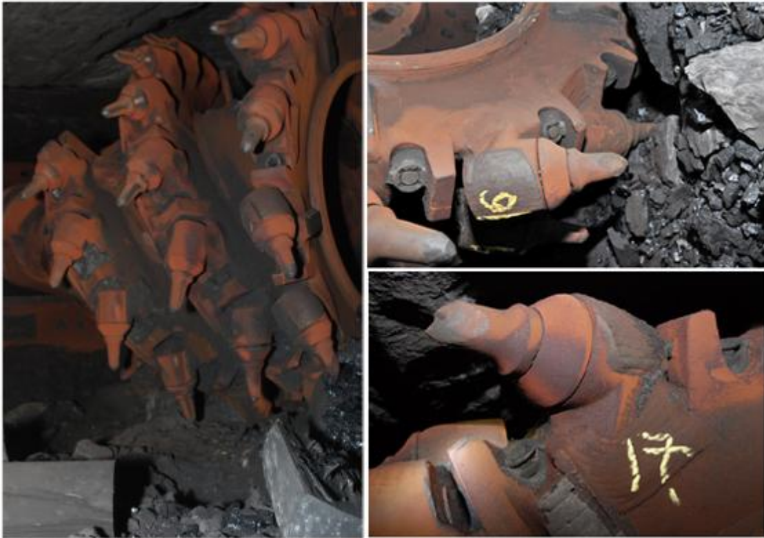
Figure 9: View of the tailgate shearer drum showing the cutter bits with tungsten-carbide tips. The bit lacing is designed to maximize the interactions of the bits as they cut away the coal and /or rock. Bits #16 and #17 are worn past most or all of their carbide tips.
