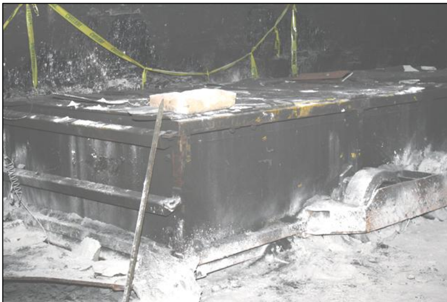
Figure 2. Strata Emergency Shelter/Refuge Chamber; #22 Headgate, approximately 20 feet north of survey station 24548 in the #2 to #3 crosscut approximately 1,060 feet outby the furthest advanced #1 face.
