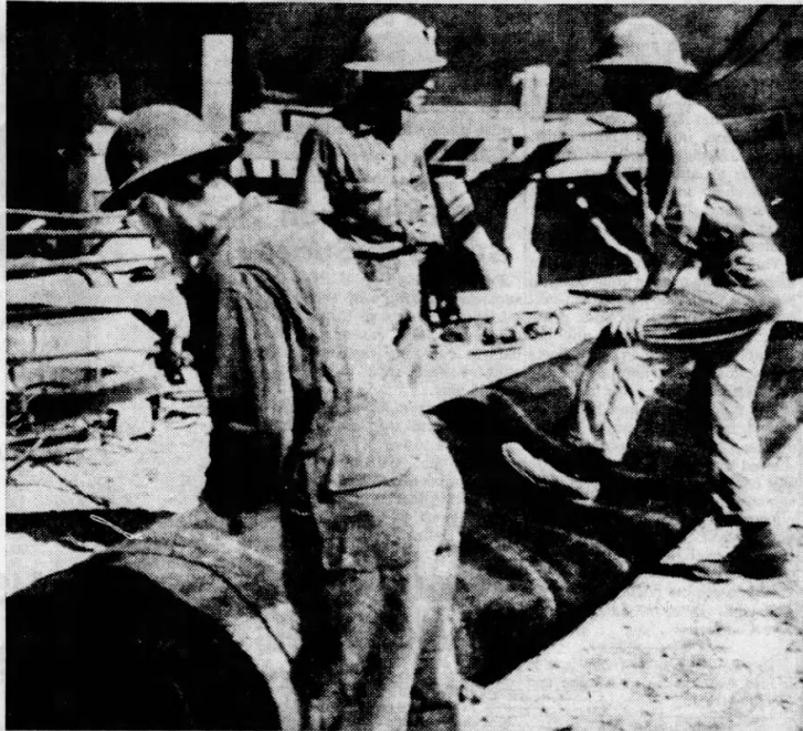
Rescue workers examine a section of the pipe used for ventilation that was damaged in an explosion in the Texas Gulf potash mine at
