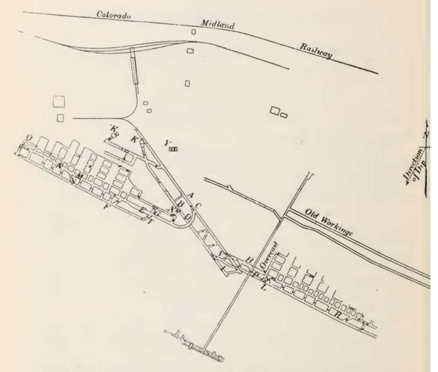
sunk from the top of the seam to the bottom of the parallel air course, and the right entry is driven to the west boundary line. At 250' from the slope the right entry runs on the strike of the seam and a double parting about 13' wide and 100' long is constructed for the purpose of facilitating the haulage. This is shown at the point E on map.
